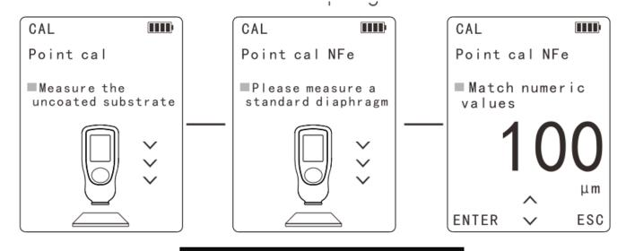
On-screen guide for calibration process
