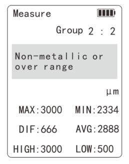
Metal putty detection to notify user of putty inside paint coatings for consideration into the thickness values.
